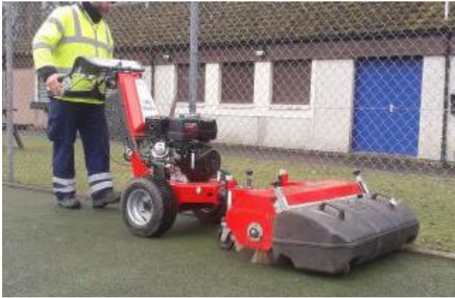
Weed brush attachment on 2 wheeled tractor
